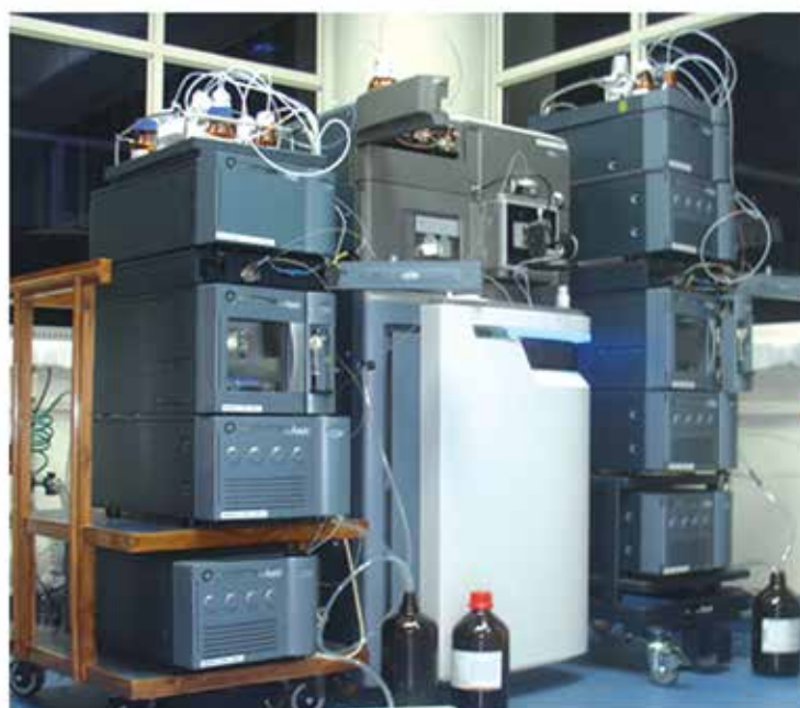
Synapt G2 HDMS mass spectrometer (middle) with 1D NanoACQUITY UPLC on the left and 2D NanoACQUITY UPLC on the right.
